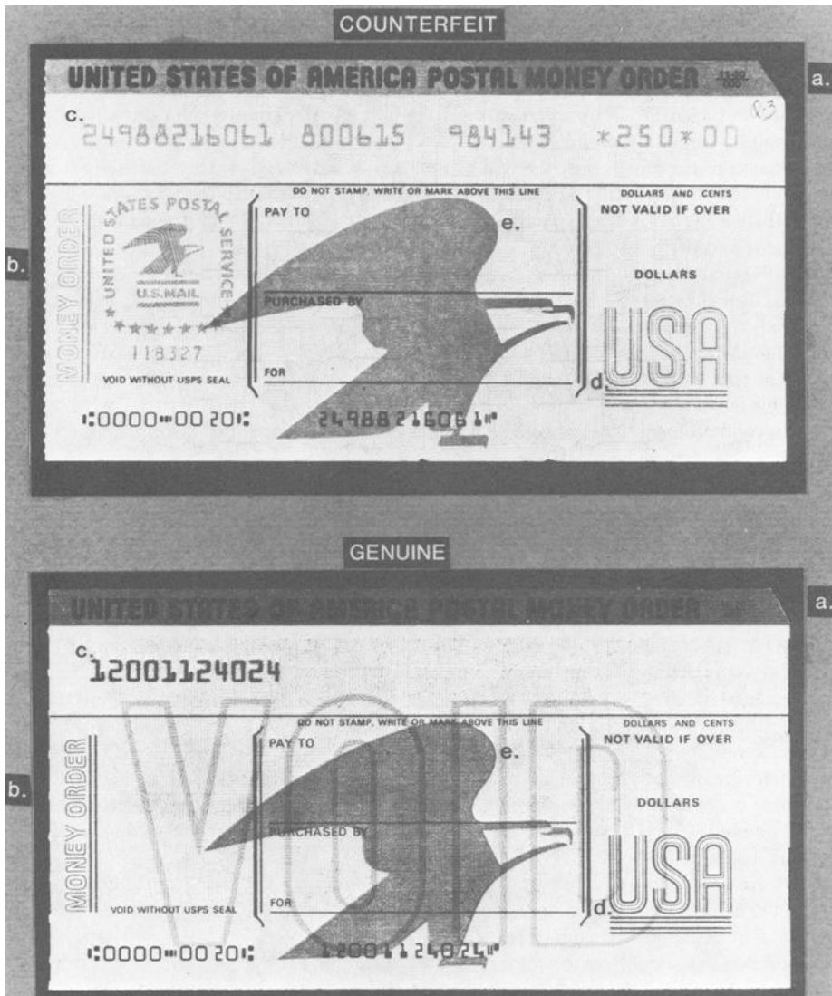
FIG. 1—Genuine and counterfeit U.S. Postal Money Orders showing: (a) orders are not trimmed completely, (b) perforations are the wrong size, (c) carbon impression is the product of a dot screen printing process, (d) fine printed lines show a broken appearance, and (e) absence of ink squeeze is apparent along the margin of the eagle's wing.
